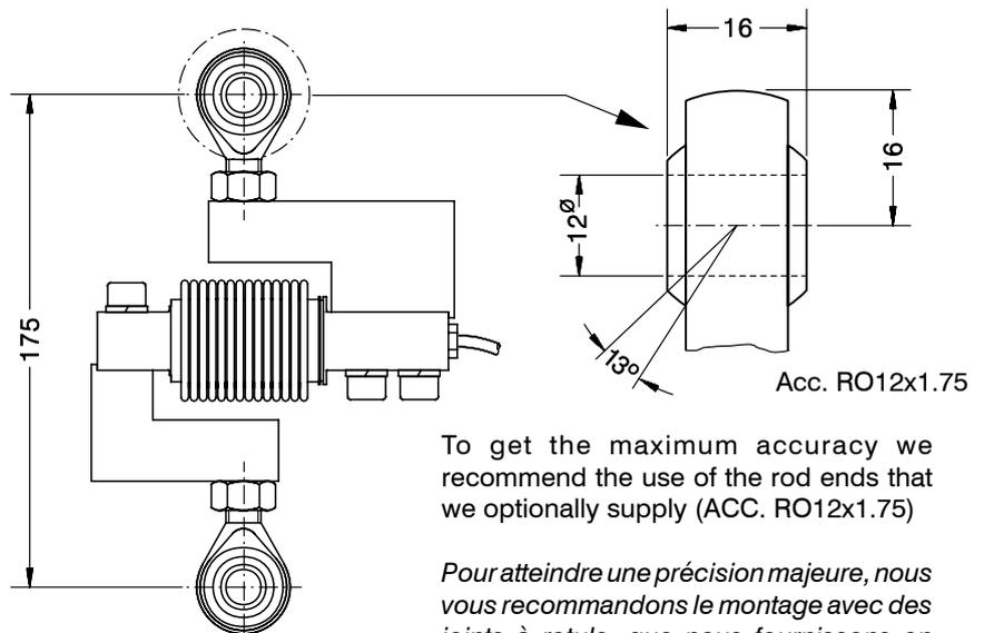
To get the maximum accuracy we recommend the use of the rod ends that we optionally supply (ACC. RO12x1.75)
